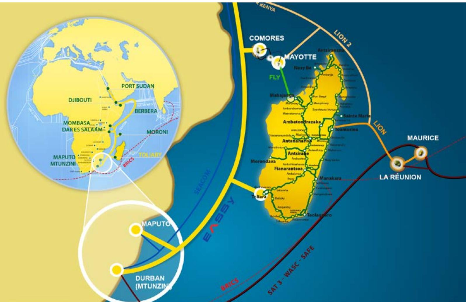
Telma has deployed wholesale solutions in Madagascar. This portfolio comprises an international connection via the **submarine cable, EASSy** (which Telma is a major investor in); a national transmission via the National Backbone in optical fiber; and network access (FO/ASDL/SDSL/WLL).
